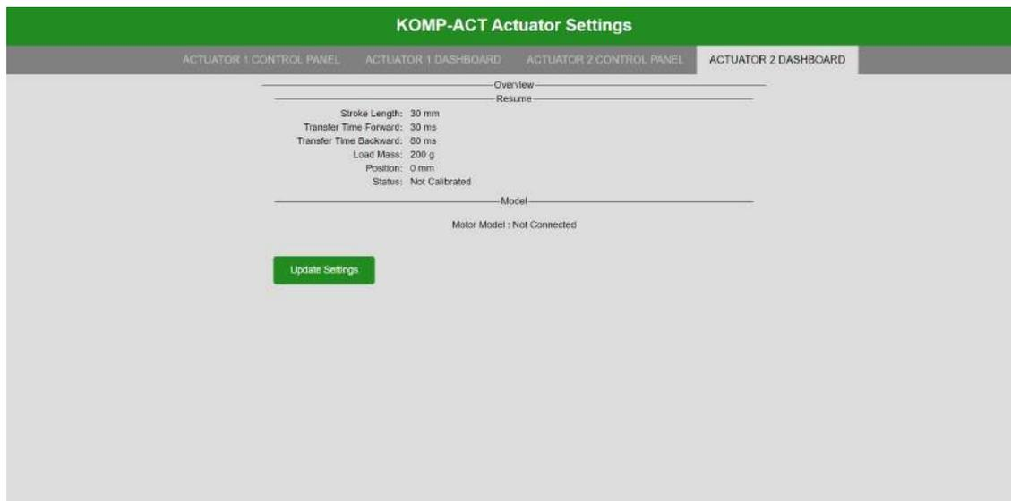
Figure 8-5 ACTUATOR 2 DASHBOARD tab of KOMP-ACT's end-user interface
