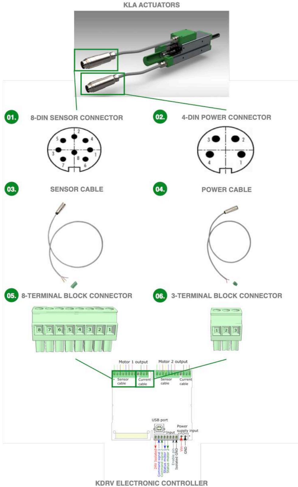
Figure 10-2 Assembly of the cables and connectors on KOMP-ACT's product line
