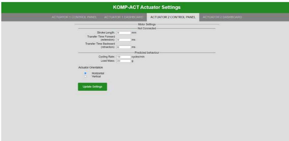
Figure 8-4 ACTUATOR 2 CONTROL PANEL tab of KOMP-ACT's end-user interface
