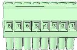
Figure 7-7 Scheme of the sensor connector on the electronic controller side
