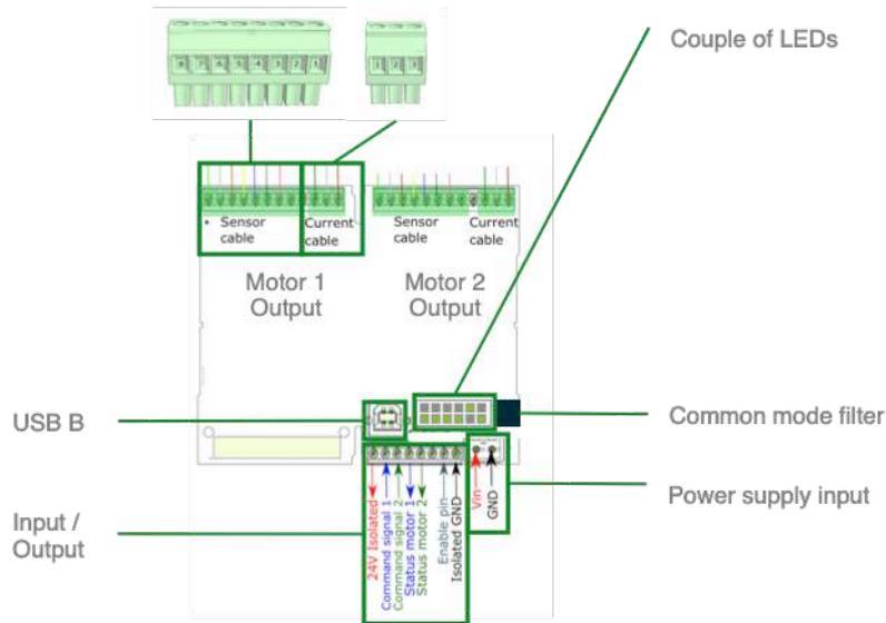
Figure 7-3 Connection scheme of KOMP-ACT's electronic controller, KDRV-1-MK-X-X
