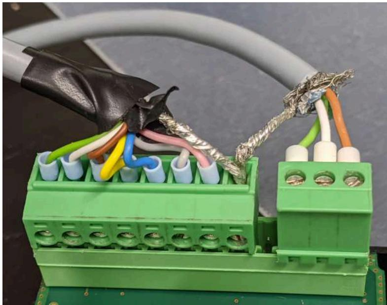
Figure 7-6 Picture of the expected motor cable connections
