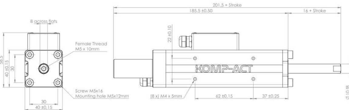
Figure 5-1 Mounting interface of KLA-40-040-0F1-2
