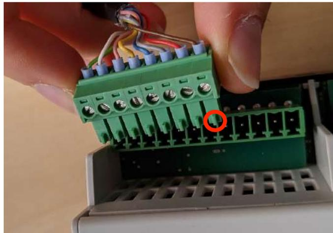
Figure 7-8 Picture showing how the board connector can be plugged, notice the small step (circled) on each connector's leg
