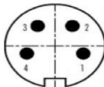
Figure 10-6 A 4-DIN power connector used in conjunction with KLA-PWR-X-03-HF-A power cable
