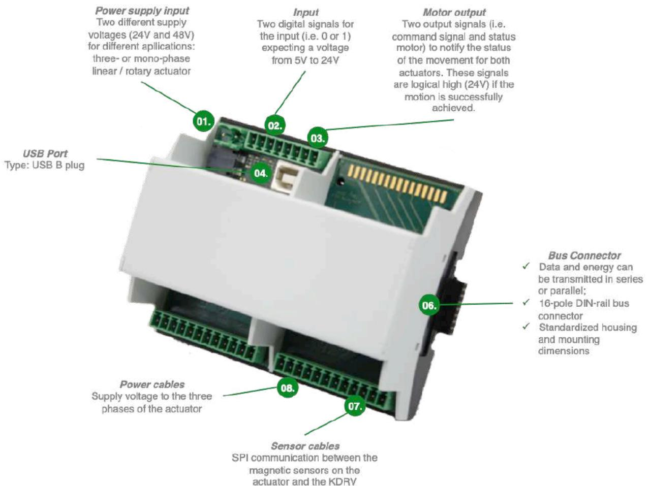
Figure 7-1 Picture of KOMP-ACT's electronic controller, KDRV-1-MK-X-X
