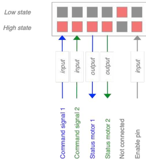
Figure 7-4 Description of the LEDs on KOMP-ACT's electronic controller, KDRV-1-MK-X-X
