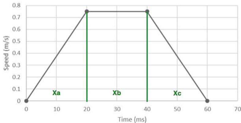
Figure 9-2 Trapezoidal profile for a specific example of 60ms stroke
