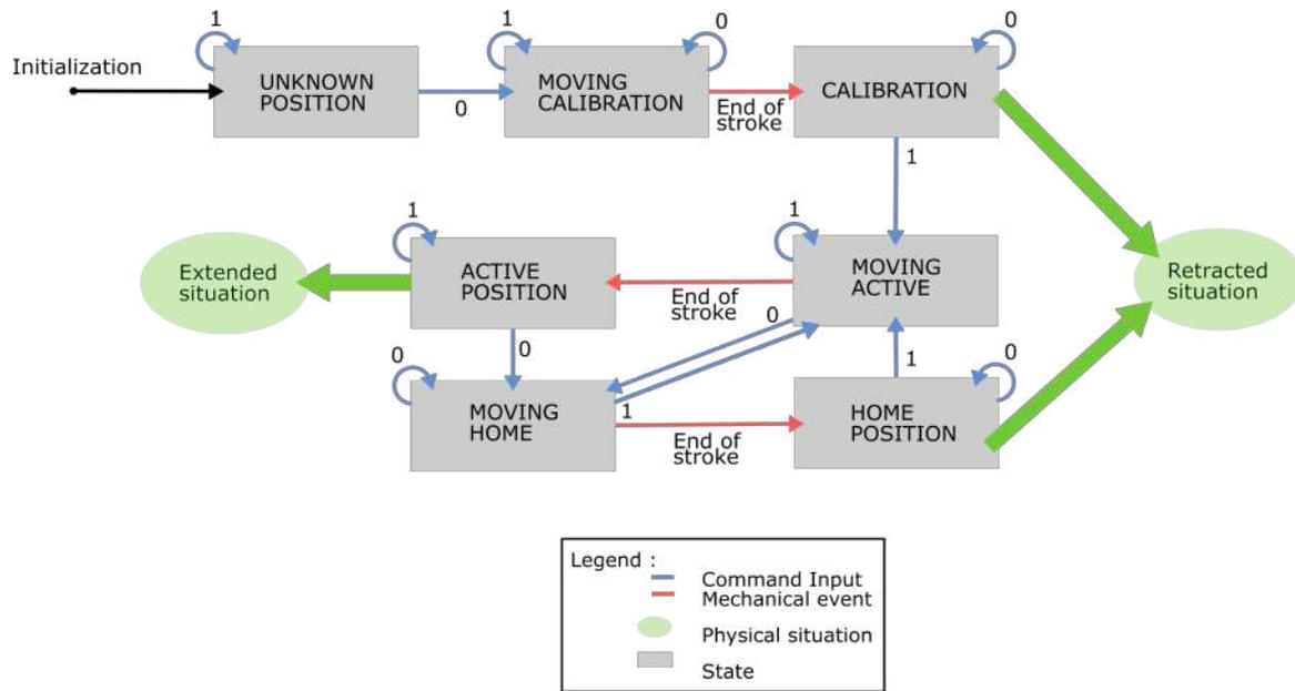
Figure 9-1 State machine of KOMP-ACT's complete solution
