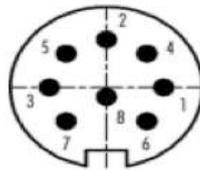
Figure 10-5 A 8-DIN sensor connector used in conjunction with KLA-SNR-X-03-HF-A sensor cable
