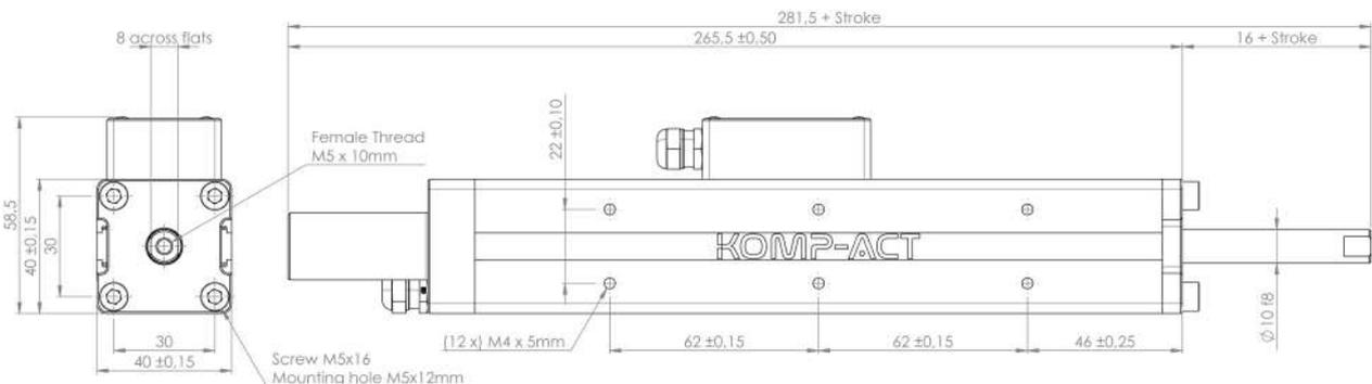
Figure 5-2 Mounting interface of KLA-40-040-0F3-2
